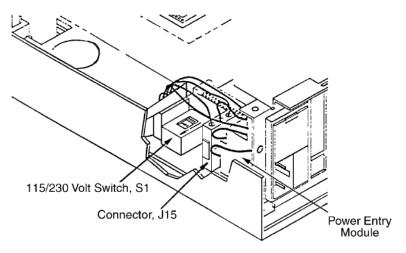
Figure 1-2 Setting Line Voltage
