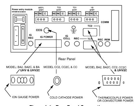
Figure 1-4 Rear Panel Connections
