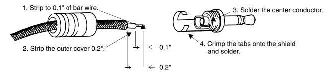
Figure 1-6 Assembling the Cable
