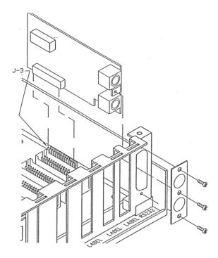
Figure C-1 Installing the Serial Communication Board
