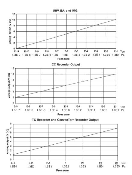
Figure 2-1 Standard Recorder Output Characteristics
