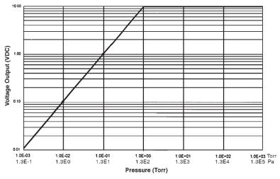
Figure 2-2 Optional Linear Recorder Output Characteristics
