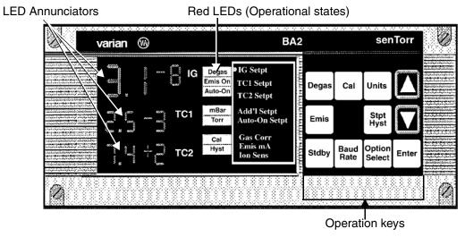
Figure 1-1 senTorr Gauge Controller Front Panel
