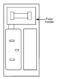
Figure 3-1 Power Entry Module
