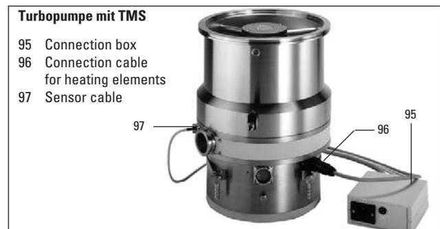
The Temperature Management System (TMS) consists of a controllable heating system which is fitted in the fore-vacuum part of the turbomolecular pump. Heating to a maximum of 90°C prevents the condensation of process gases or by-products in this part of the pump.
