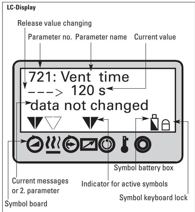
The LC display enables the representation of various operating conditions. The influence on the vacuum components and their operational behaviour is controlled via parameters; this means via specific numeric combinations to which are assigned functions. The parameters which can be selected are explained in the parameter lists in Sections 5.2. and 5.3.
