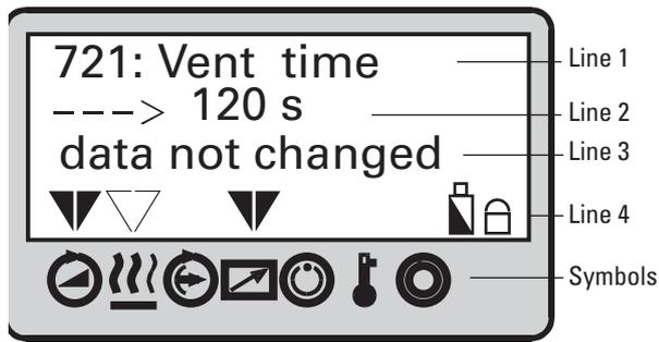
The display of the functions is shown via a four line LC display. In normal operations a specific function is assigned to each line:
